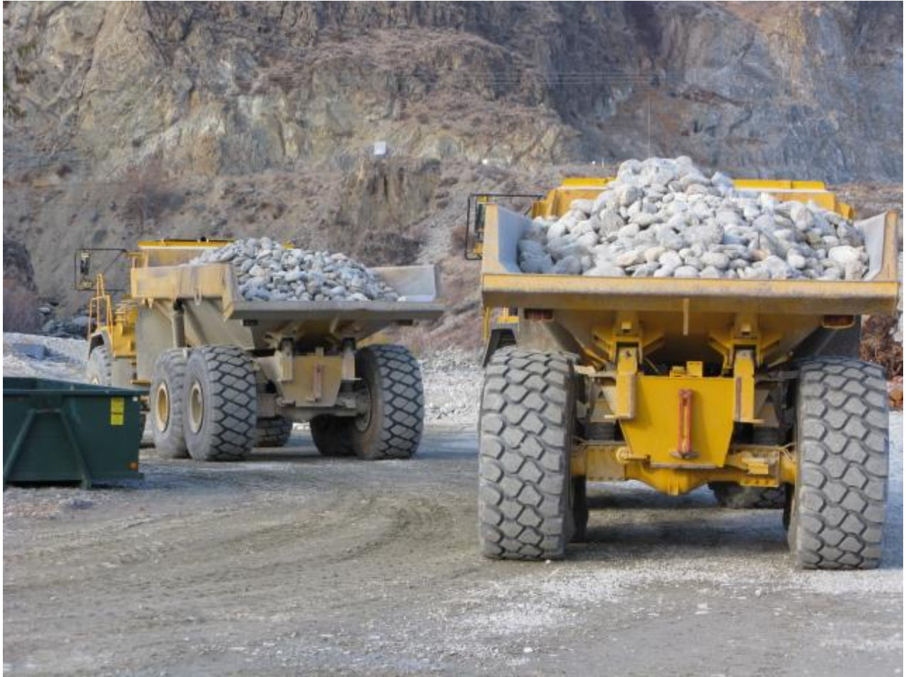
6X6 Off-road dump trucks hauling riffle mix to the habitat channel. 11/5/08
